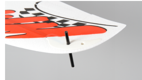
31.Reserve two mounting holes on left and right wing tip, consumers can choose the suitable hole they think, then bond with glue
