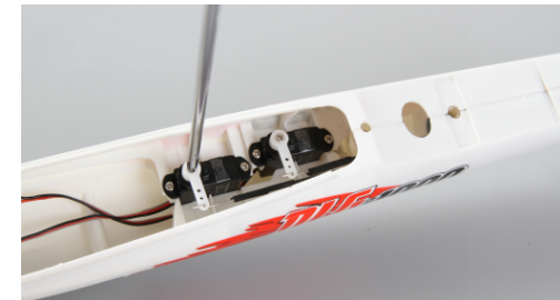
10. Cross the pushrod into carbon tail rod of fuselage and install it on the adjuster and rudder servo horn, then fixed with screw, and make sure to keep the rudder in the same horizontal line.
