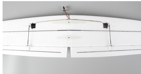
17. Aileron connection as picture.
