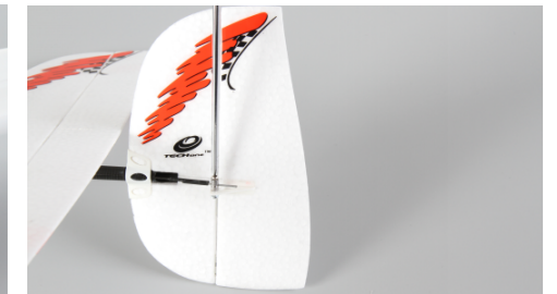
10. Cross the pushrod into carbon tail rod of fuselage and install it on the adjuster and rudder servo horn, then fixed with screw, and make sure to keep the rudder in the same horizontal line.
