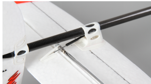
6. Cross the pushrod into carbon tail rod and install it on the adjuster and elevator servo horn, then fixed with screw, and make sure to keep the rudder in the same horizontal line.
