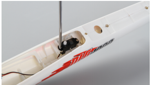
4. Insert and screw the servo into the slot on fuselage by screwdriver.
