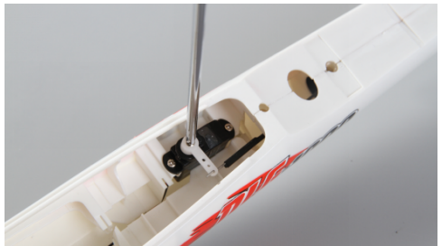
6. Cross the pushrod into carbon tail rod and install it on the adjuster and elevator servo horn, then fixed with screw, and make sure to keep the rudder in the same horizontal line.
