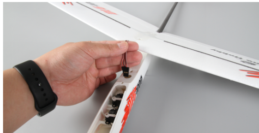
18. Cross the aileron servo into the routing hole of fuselage.
