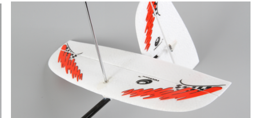
2. Install elevator on plastic plat of fuselage with screw by screwdriver.
